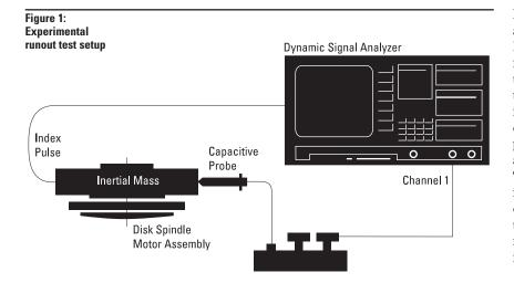
Figure 1 shows a typical test setup to measure spindle runout. The motor and spindle assembly is typically loaded with an inertial mass to simulate actual running loads. A proper load is often required for the spindle servo to maintain a constant speed.
