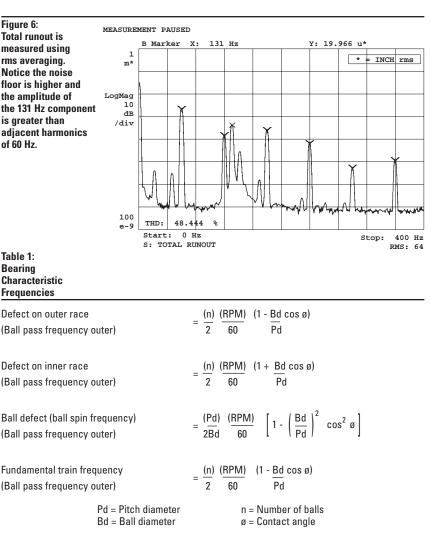
Note: for bearing spindle assemblies where the inner race is stationary, the bearing frequency can be calculated by changing the sign in the brackets or parentheses.
